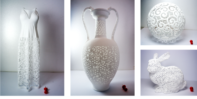
Figure 19: Prototypes printed by Stratasys Fortus 400mc and EOS FORMIGA P 110.
