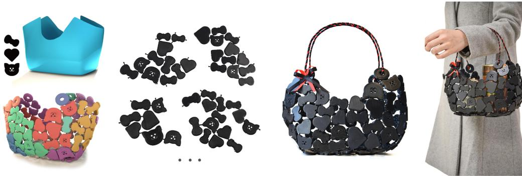
**Figure 3.12** Given a target surface and a set of user-specified tiles (top left), our method produces a dedicated packing of tiles that is optimized for fabrication (bottom left). The results are printed as independent flat patches (second column) with integrated hinges and snap-fit joints. The patches are folded and assembled into the final object (third column); in this case a functional handbag that can carry light objects.
