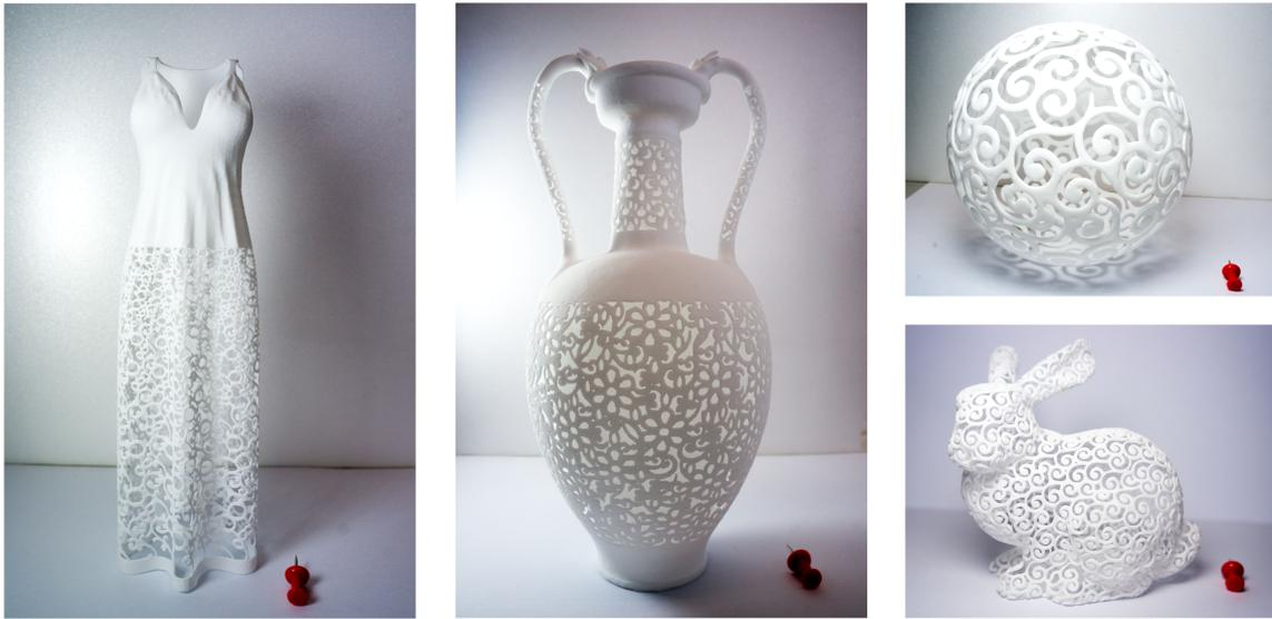
**Figure 2.19** Prototypes printed by Stratasys Fortus 400mc and EOS FORMIGA P 110.
